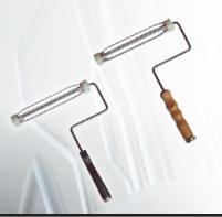
Heavy-duty 8mm (5/16") chrome-plated steel shank, reduces bending when using with an extension pole. Heavygauge 3.8mm five wire cage assembly. Available in both natural hardwood and injection-moulded plastic handles with metal insert or grommet for extra strength. Threaded for use with extension poles.
