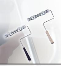
Heavy-duty 8mm (5/16") chrome-plated steel shank, reduces bending when using with an extension pole. Two tension bends on five wire cage assembly to prevent refill creeping. Available in both natural hardwood and injection-moulded plastic handles with metal insert or grommet for extra strength. Threaded for use with extension poles.
