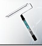
Sturdy 6.4mm ( $\frac{1}{4}$ ") galvanized steel shank. Two tension bends on five wire cage assembly to prevent refill creeping. Available in two unique Simms comfort design injection-moulded plastic handle designs. Threaded for use with extension poles.
